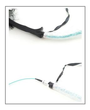
Remove bubble wrap by pulling towards end where bubble wrap is sealed.
