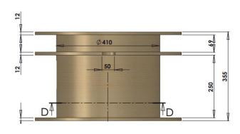
The new reel (POP-UP II) has the same dimensions and mechanical stability as the SIZE II reel – on top of that, it has the added a feature of **easy disassembly** after use, as shown in the following pictures:
