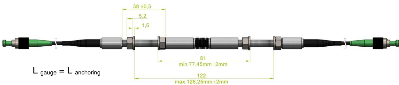
Figure 1. Schematic representation of the SC-01 gauge and anchoring length.
