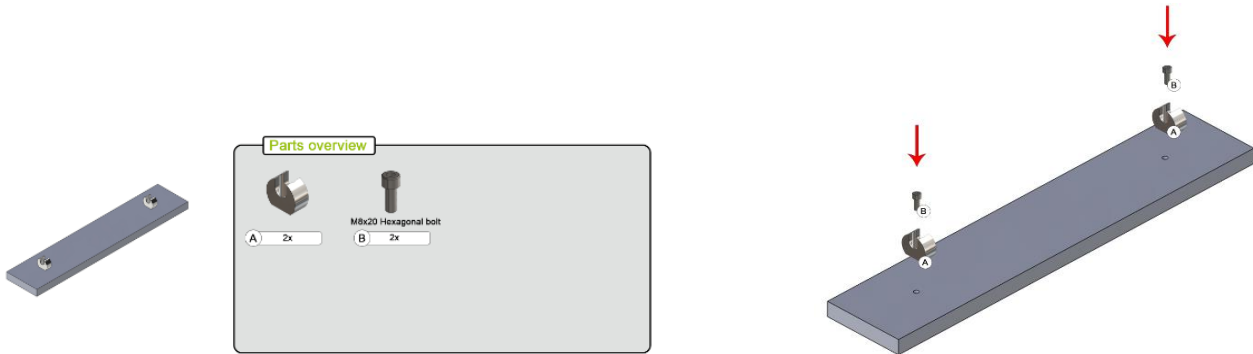
Figure 4: Mechanical installation of the mounting brackets.
