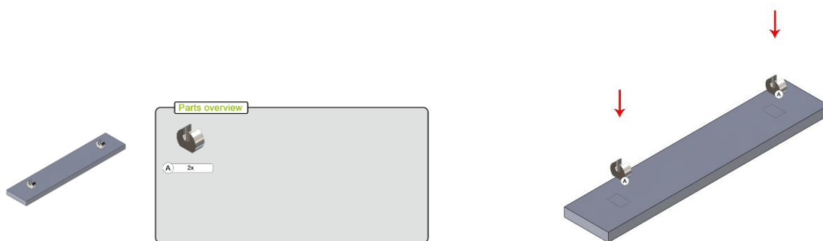
Figure 5: Chemical installation of the mounting brackets.
