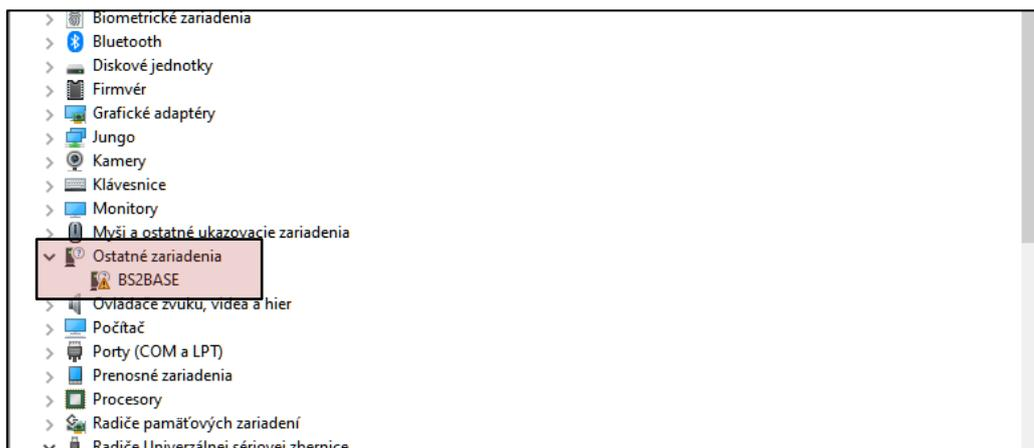
**Figure 1:** Unknown hardware detected by the OS after connecting the unit to the PC for the first time.
