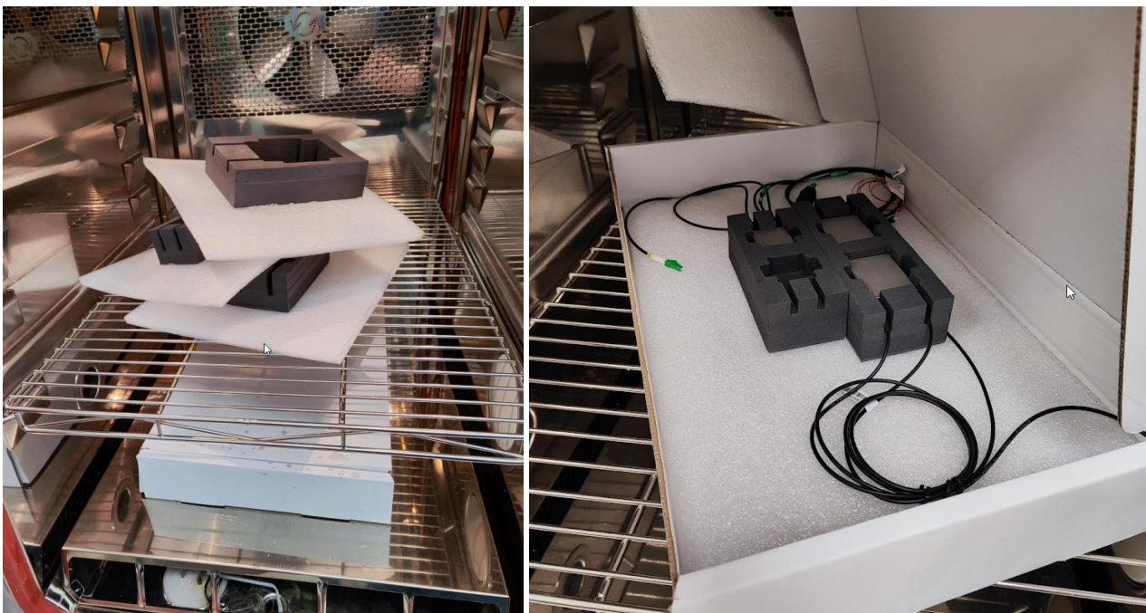
Figure 2 Testing foam and cardboard box in climatic chamber
