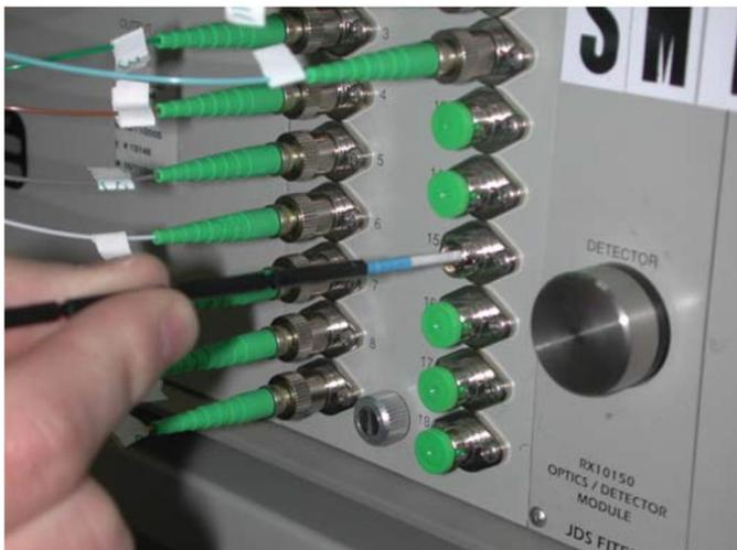
**NOTE:** OPTIPOP Stick Cleaners remove debris from the ferrule tip inside the adapter as well as the internal wall of the split sleeve
