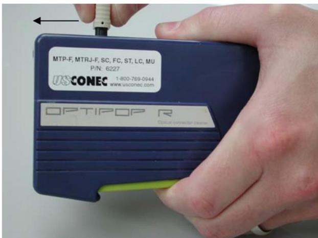
3. Release the green lever of the cassette to cover the cleaning material.
