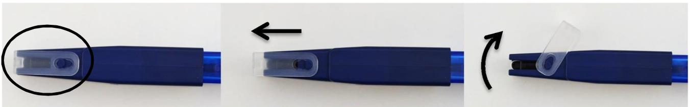
2. Remove dust cap from the MXC plug connector.
