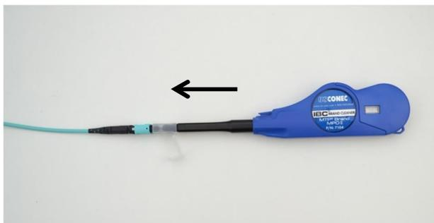
***NOTE:** The MTP I.B.C. cleaner dust cap simulates an MPO/MTP adapter. Insert the connector into the cap with the key of the connector matching the keyway of the cleaner.*
